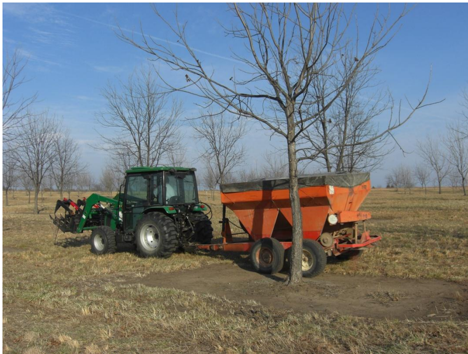
Fig. 1. Wagon type tractor pulled fertilizer spreader in action.
